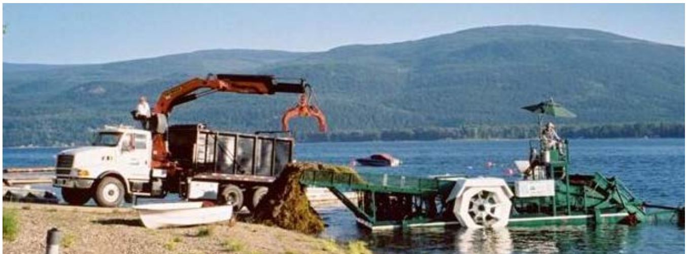
CRANE TRUCK LOADING HARVESTED MILFOIL
