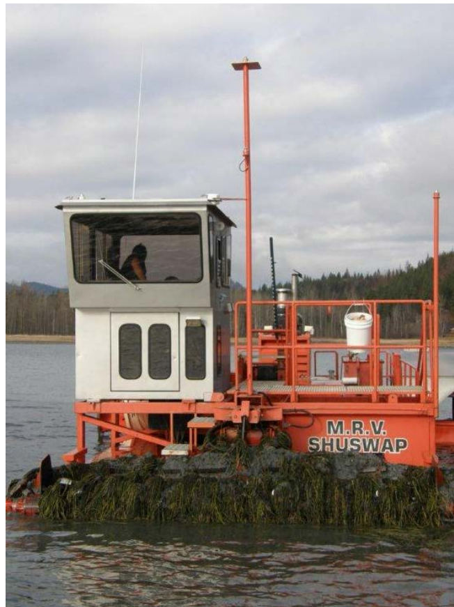
THE 'M.R.V. SHUSWAP' MILFOIL ROTOTILLING VESSEL
